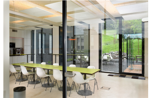
The cafeteria is housed in the structure linking the two buildings. Eighteen PADs were also installed on the ceiling here to enhance the room's acoustics. (Photo: Jean-Luc Grossmann/photopulse)
