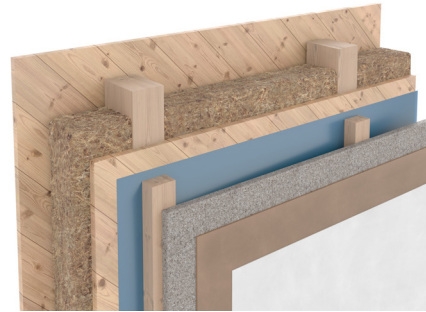
The supporting structure and large parts of the façade consist of untreated wood, a material that can be reused or composted after the building is dismantled. Rendering: Werner Sobek with Dirk E. Hebel and Felix Heisel
